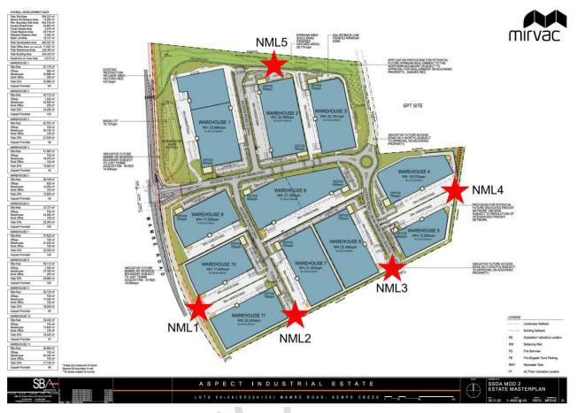
Figure 6: Noise Monitoring Locations Plan
