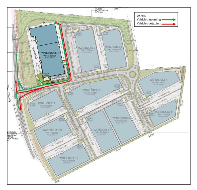
Figure 7: Ultimate Access Construction Vehicle Access Route
