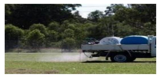
Figure 4: Boomless spray nozzle attached to a truck
