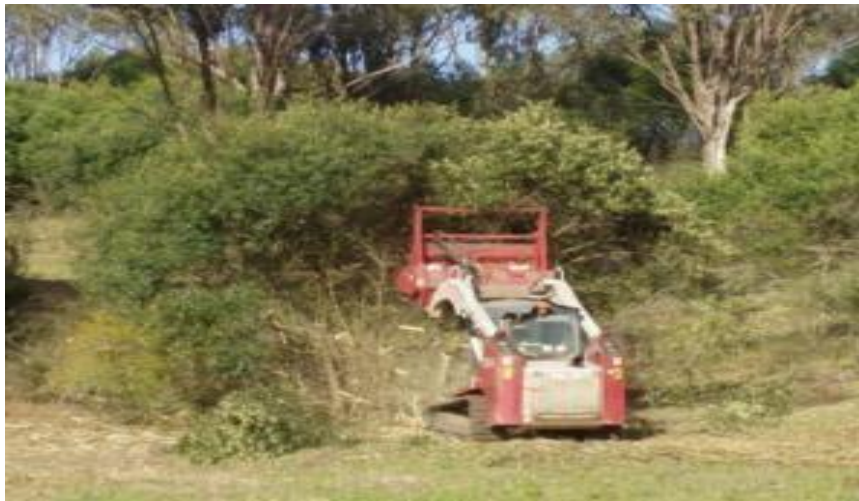
Figure 10: Triter machine mulching African Olive
