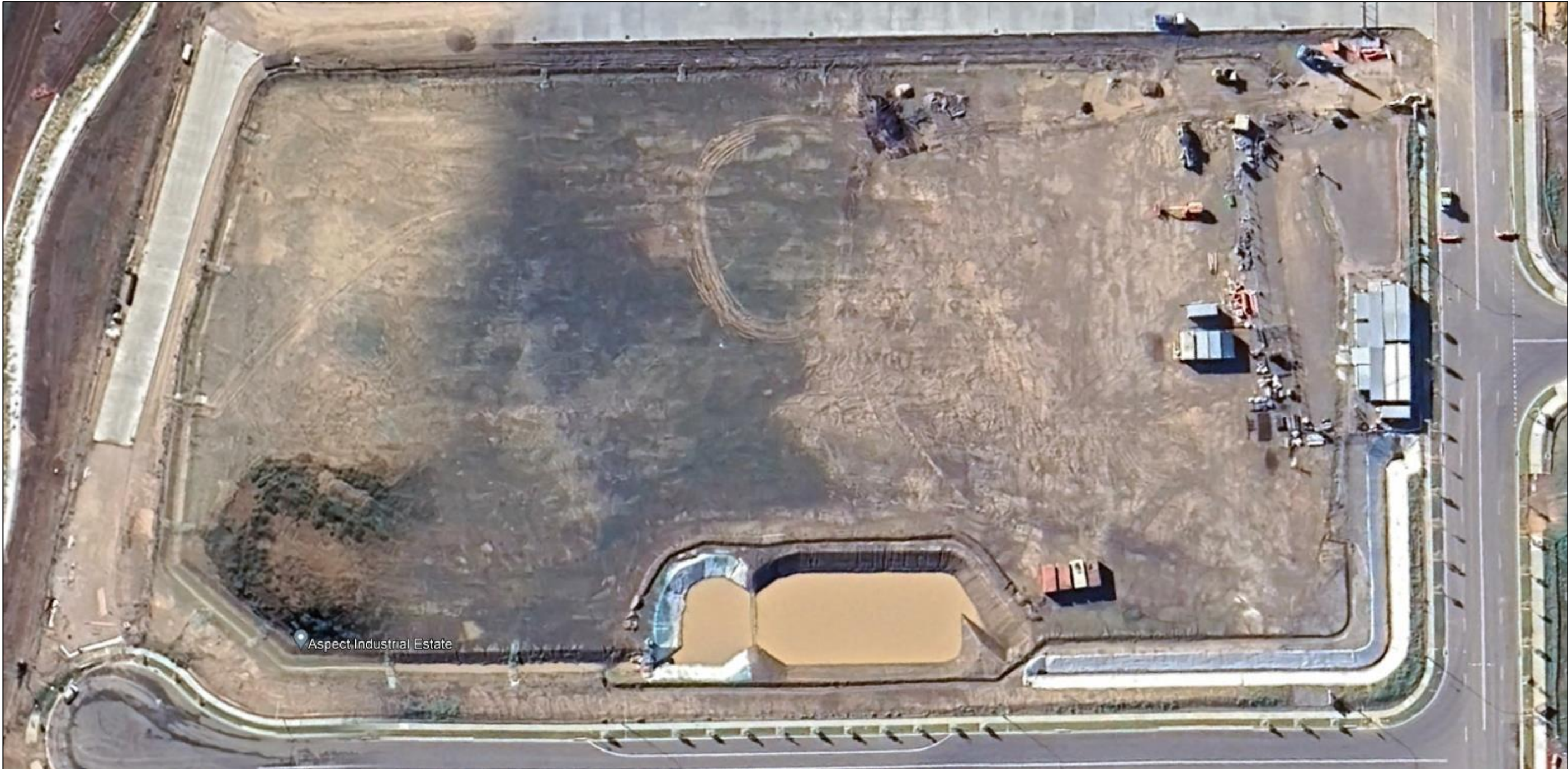
Aerial View of the current construction and erosion and sediment controls occurring on the AIE site – Aerial imagery from Google Earth: June 2024
