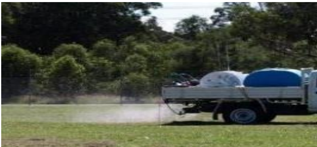
Figure 5: Boomless spray nozzle attached to a truck
