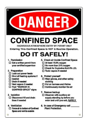
**Example C:** Mobile Confined Space Warning Sign that can be established in a prominent position adjacent the Confined Space.
