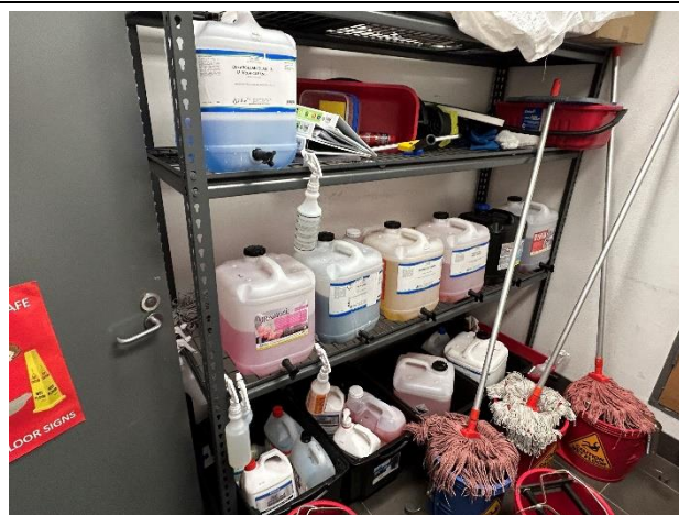
Photo 06. Chemicals stored without appropriate secondary containment in Level B1 Cleaners Store Room.
