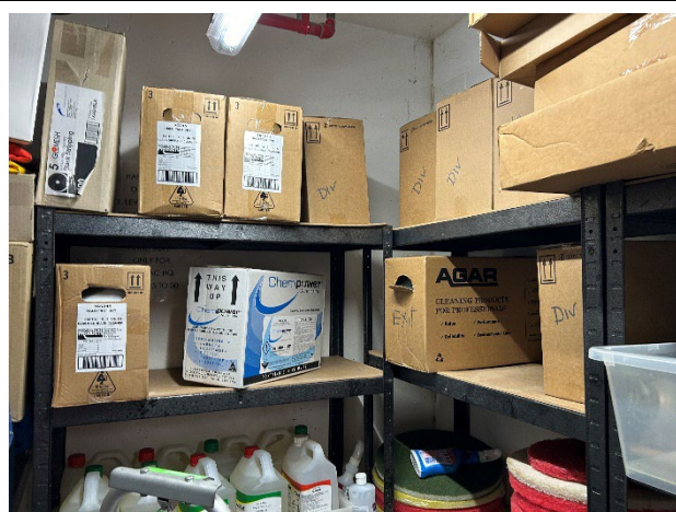
Photo 03. Chemicals stored without secondary containment in the Level B4 Store Room.
