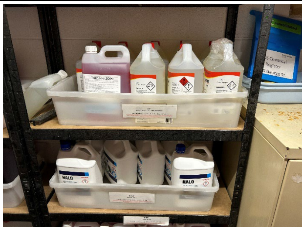
Photo 05. Class 8 and Class 3 hazardous chemicals stored together in the Level B4 Store Room.
