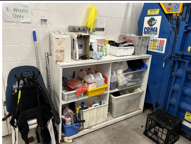
Photo 06. Class 8 and Class 3 hazardous chemicals stored together in the Level US Waste Room.
