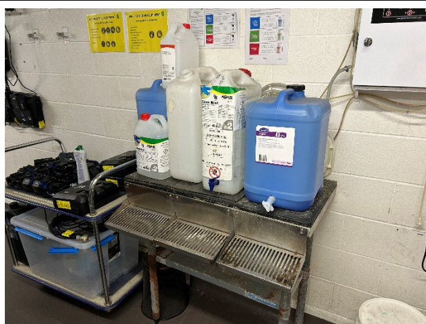
Photo 04. Chemicals stored without secondary containment in the Level B4 Cleaners Store Room.
