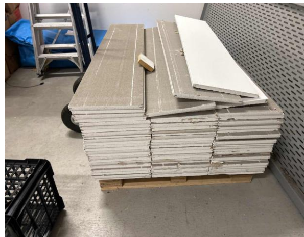
Line ID 13: Internal, L3, Lift Lobby, Stored Ceiling Tiles, Northeast of Lift, Compressed Ceiling Tiles - Suspected SMF
