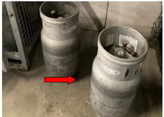
Photo 14. Inappropriately stored gas cylinders in the Greek Street Building, Dock.
