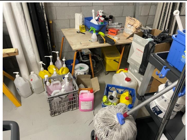
Photo 08. Hazardous chemicals without secondary containment in the Level B1 Store Room..
