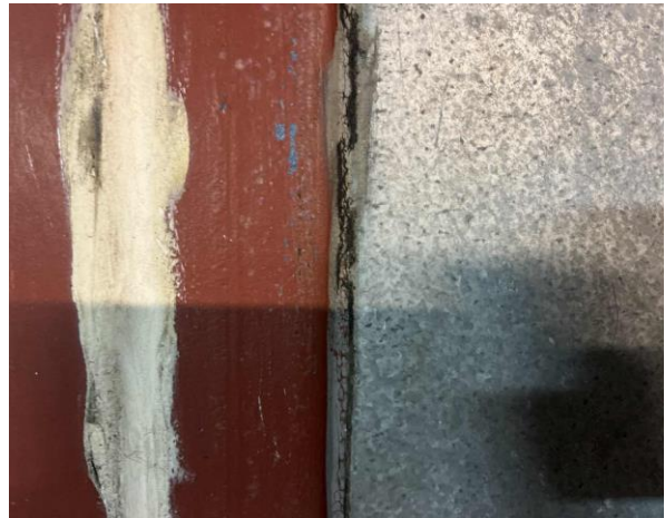
Line ID 47.1: Internal, L14, Plant Room, Air Handling Unit Panel Sealant, Mastic Sealant (Black & Dark Grey) - No Asbestos Detected
