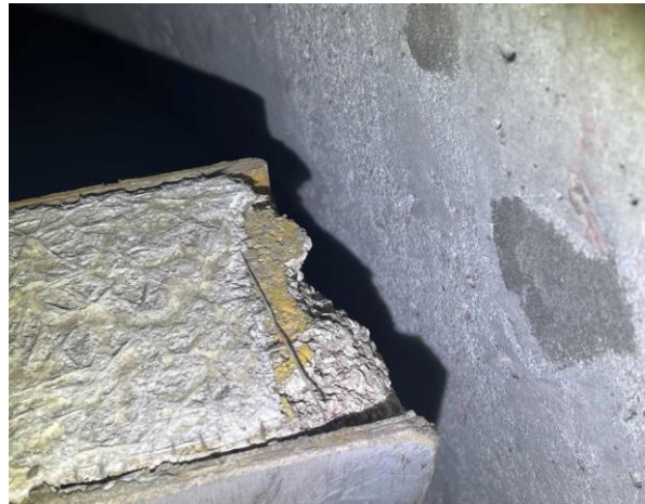
Line ID 90: Internal, L23, South Air Handling Unit AHU-7, To Hatch Door Internals to RAF6, Vermiculite - No Asbestos Detected
