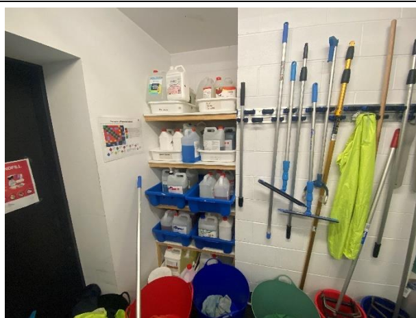
Photo 02. Level 9, Cleaners Store Room, class 3 flammable liquids stored above and below class 8 corrosive chemicals.
