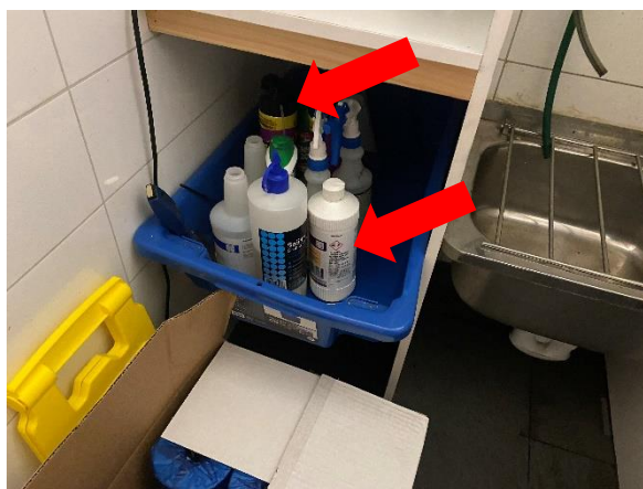
Photo 04. 4 Riverside Quay, cleaners store room – incorrect storage of class 8 and class 2.1 chemicals.
