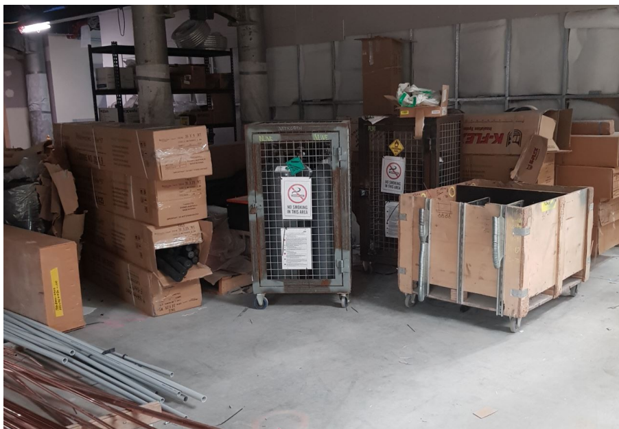
Photo 9: Inappropriate storage of gas cylinders near combustible materials
