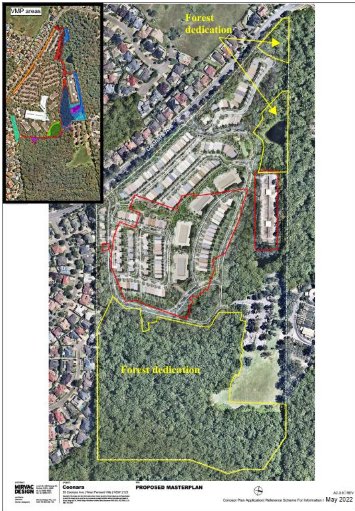
Figure 1: Concept Masterplan showing the proposed development footprint, bushland to be retained and managed under a VMP (inset), and bushland to be dedicated to State Forests (yellow). Impact area already assessed in the Demolition BDAR is outlined in red. VMP areas by Cumberland Ecology.
