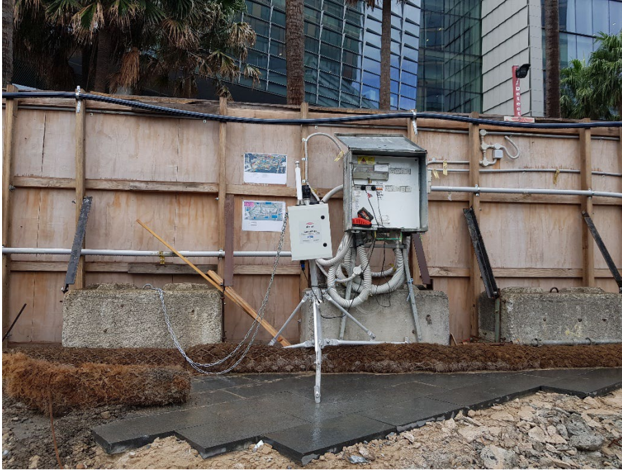
Photo 27: Continuous particulate (PM 10 ) dust monitor in the south-western corner of the site. 23/01/24
