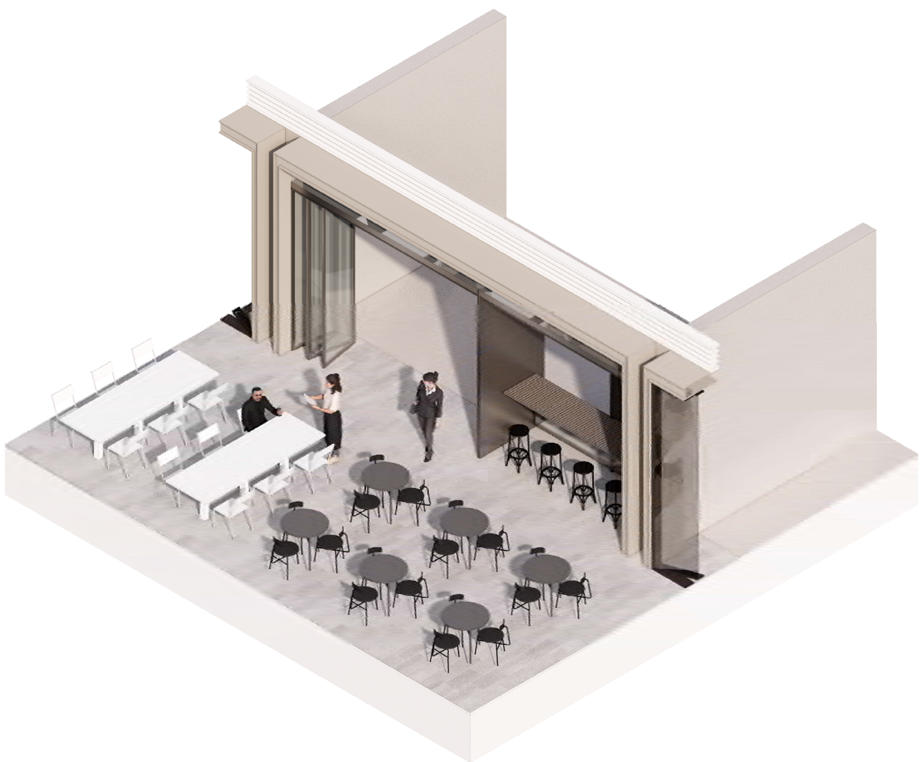
Typical Sliding Operability with Integrated Bar Seating - Illustrative Axonometric (NOT TO SCALE)
