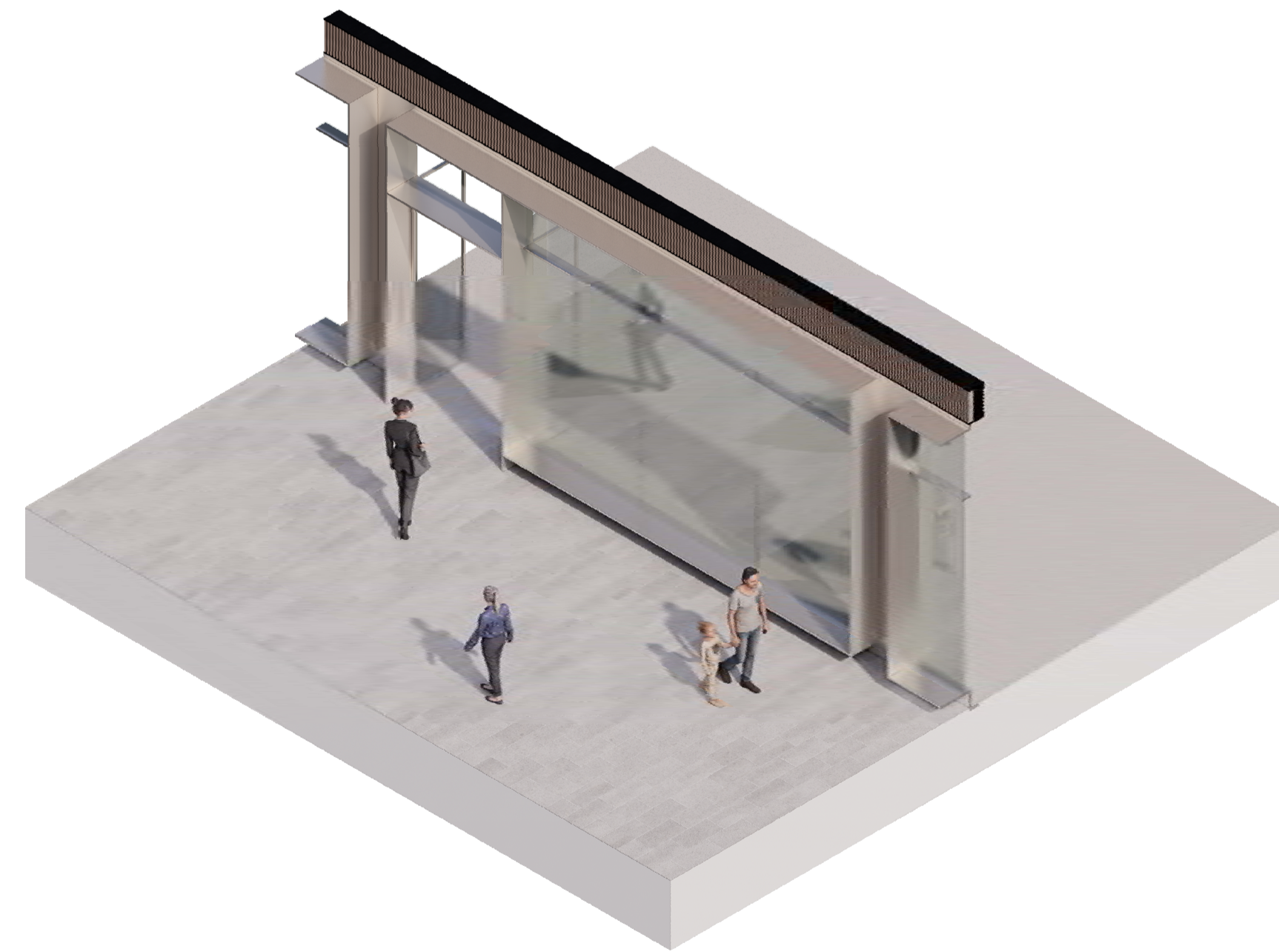
Typical Fixed Panelling with Swing Door - Illustrative Axonometric (NOT TO SCALE)
